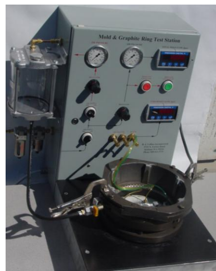
Figure 3 Accu-Test™ Billet Mold Testing System
