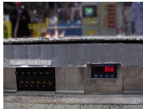
Figure 6 Typical Accu-Set™ Mass Flow Mold Calibration Installation
