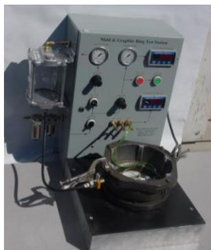
led the way in developing a means of measuring the casting characteristics of a graphite ring to insure better performance (Figure 5). This is the first time such equipment has been available.
