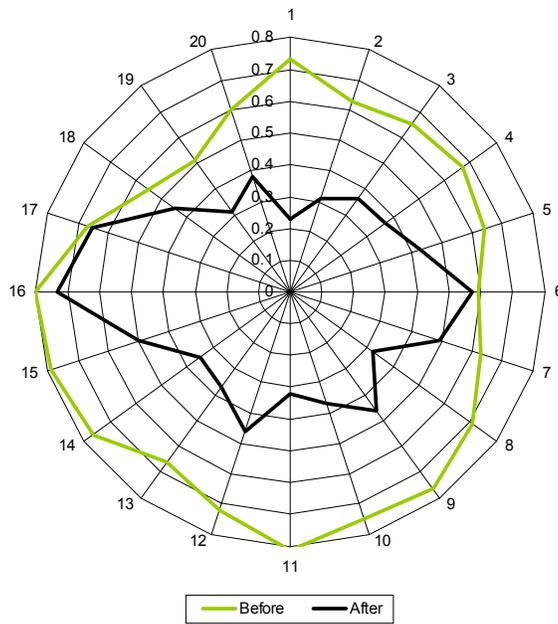
**Figure11.** Ring permeability before and after being in production.
