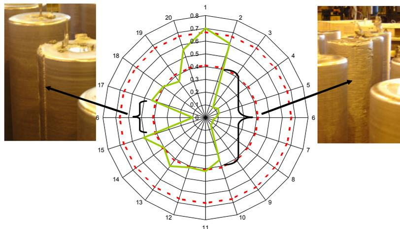
**Figure 9.** Billet surface defect versus uniformity flow.
