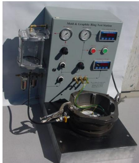
**Figure 2.** RJ Collins graphite ring tester.
