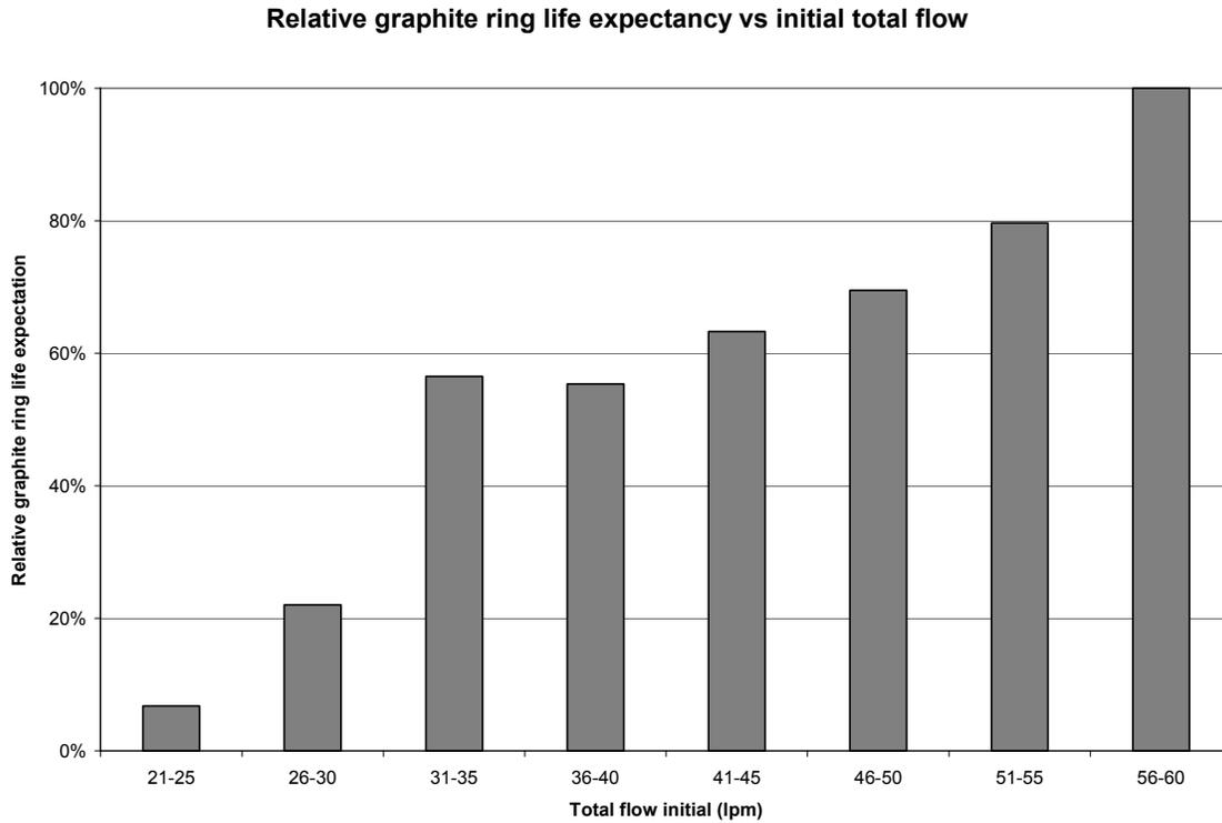
**Figure 7.** Initial total flow impact on graphite life expectancy.
