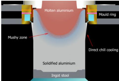
**Figure 4.** Casting mold and apparatus.
